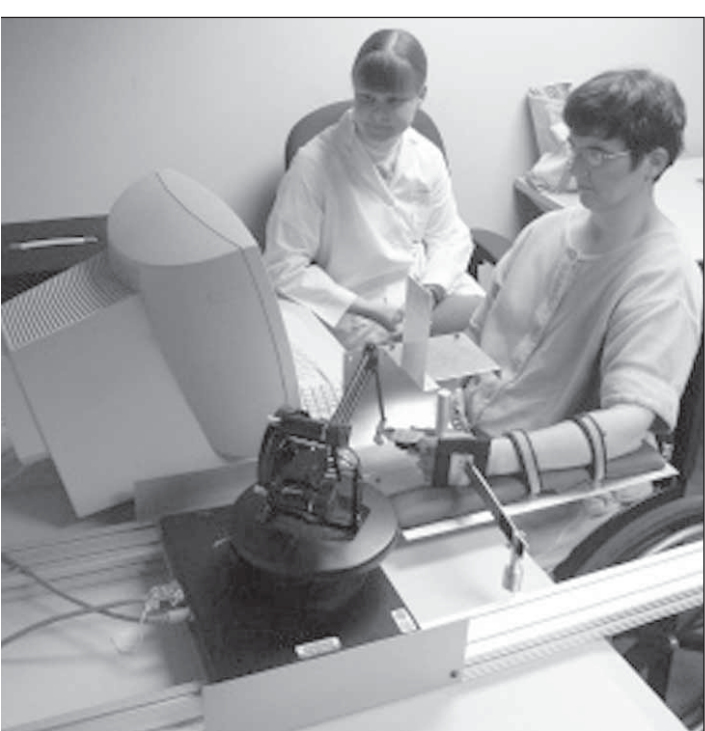
The Matsuoka lab has constructed a robotic environment to combine the repetitive movements of robotic therapy with visual feedback distortion.
