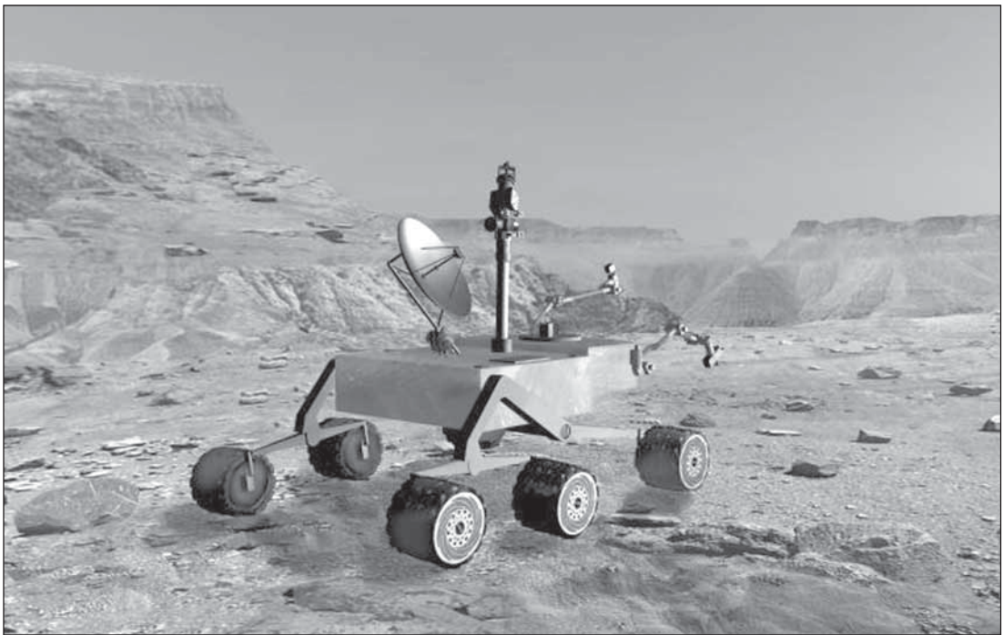
Courtesy of www.nasa.gov A NASA rover, scheduled to go to Mars in 2009, will be equipped with a neutron activation apparatus to detect hydrogen-rich water molecules.
